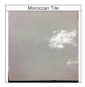
The Moroccan Tiles were of an encaustic design with a noticeable amount of lightly bound 'release agent' on the rear of the tiles. This surface contamination was successfully removed via brushing the rear surface with a stiff nylon brush which revealed the true tile body.
